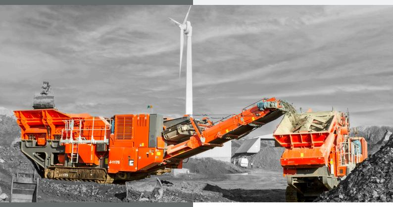
The Finlay® J-1175 electric jaw crusher has been designed to meet the needs of customers for whom electricity is the preferred power source. The intelligent and flexible design of the power pack enables the machine to be connected directly to the grid or a genset electrical power source.
