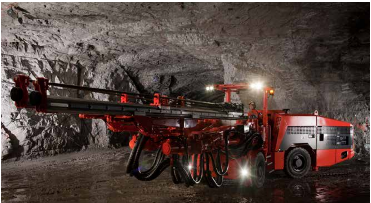
1. SANDVIK DT621 - TUNNELING DRILL
