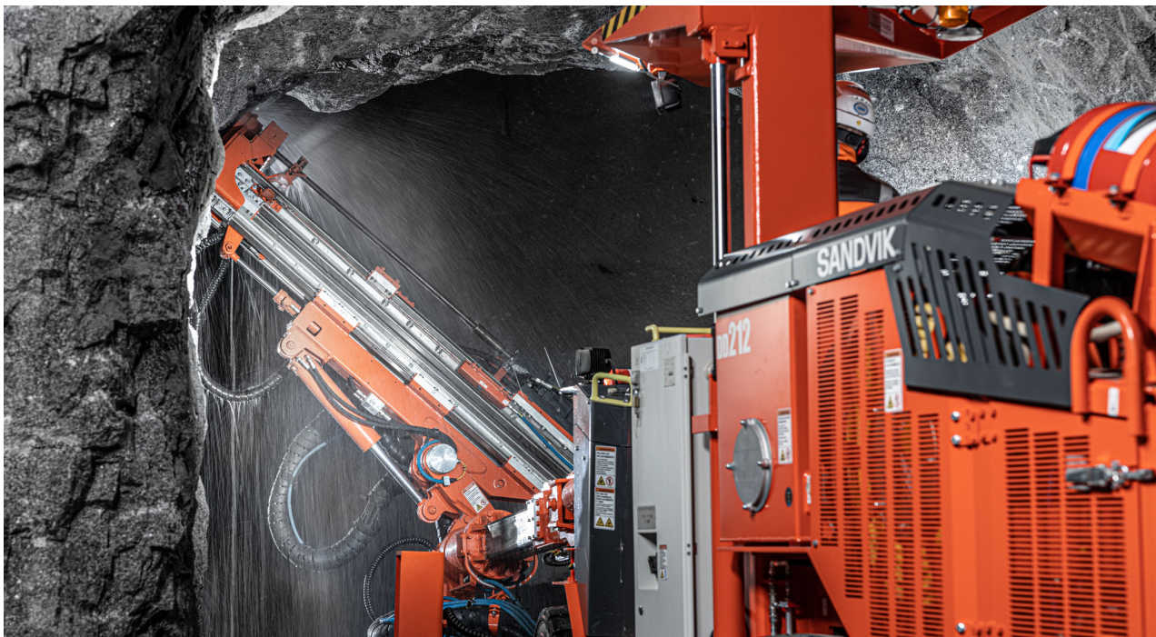
1. SANDVIK DD212 - NARROW VEIN DRILL
