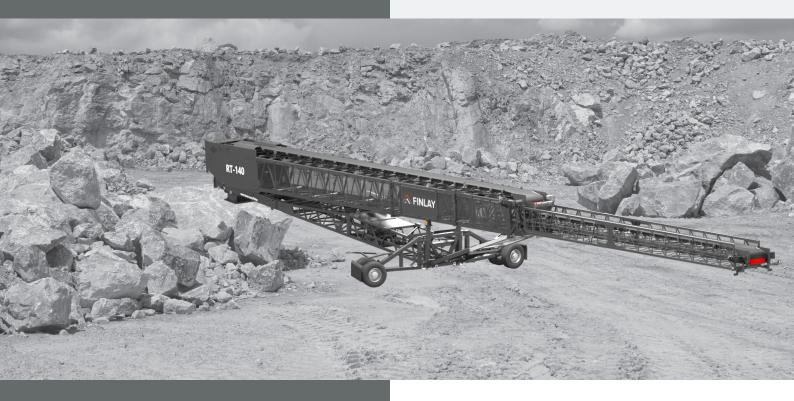
The Finlay<sup>®</sup> RT-140 telescopic conveyor is essential for producers who want to produce a consistent quality product and reduce segregation, degradation, compaction and contamination of material in the stockpile.
